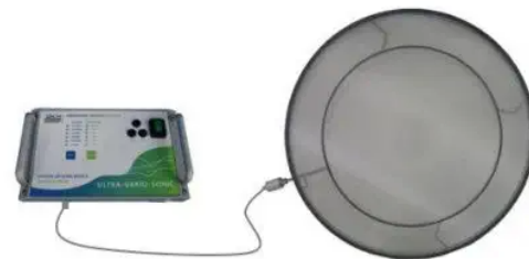
Ultrasonic generator with sound-transmission ring bonded to the screen
