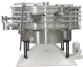
GKM KTS tumbler screener, stainless execution
